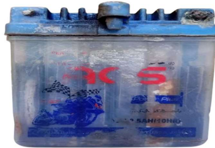
Fig. 6. Lead Acid Battery
