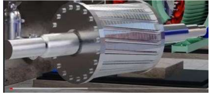
Fig.2. Synchronous reluctance motor rotor
