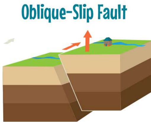
Figure 3(d). Oblique-Slip Fault Rupture
